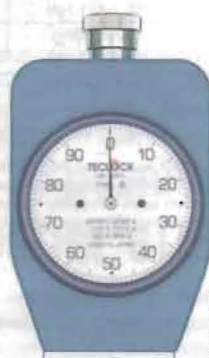
GS-709N Type A Durometer General rubber Soft plastic
