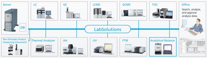
Integrated Management of Analytical Data via a Network System Using LabSolutions
