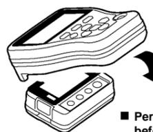
Place the logger and collector so that their IR ports are aligned.
