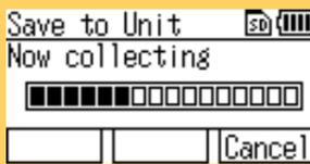
The display on the left is shown during data collection. When you want cancel data collection part way through: Press the **F3** button to return to the top display.
