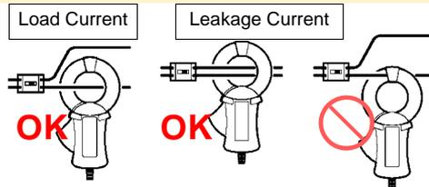
9675 Clamp On Leak Sensor
