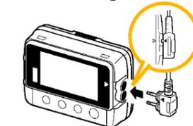
Align the triangles on the plug body and in front of the cable jacks, and insert the plug securely. (Insert the protruded parts of the connecting cable into the holes of the device.)
