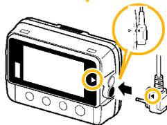
2 Connect the LR9801 Connection Cable to the logger.
