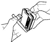
1 Install the battery in the logger.
