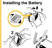
Press the PUSH tab as shown, and pull the battery cover back.
