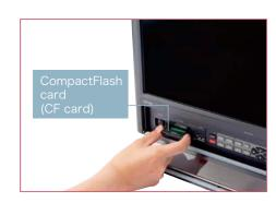
Front CompactFlash card slot. Data can be backed up "as is" to a PC.
