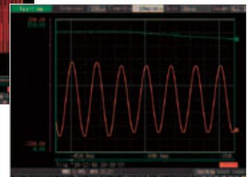
**3** Measure the phase voltages for all three phases of a three-phase motor simultaneously.
