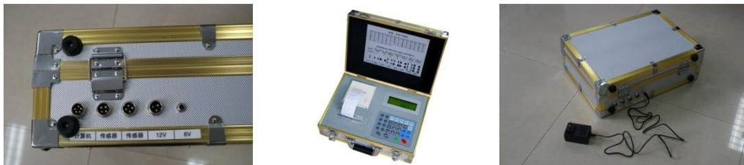
It is used to inspect the overload of the vehicle on the road in dynamic or static. It could weigh the dynamic vehicle in low precision or static vehicle in high precision.
