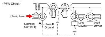
If leakage is occurring, investigate by lumped measurements (clamping all lines together) starting from the supply side toward the load.
