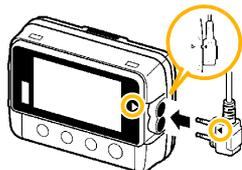
2 Connect the LR9802 Connection Cable to the logger.
