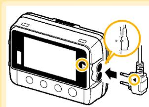
Align the triangles on the plug body and in front of the connection cable jacks, and insert the plug securely.
