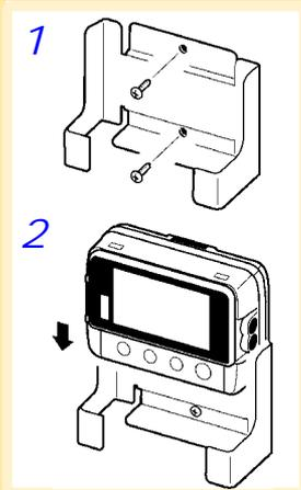
1 Mount the LR9901 to the wall using the two screws.
