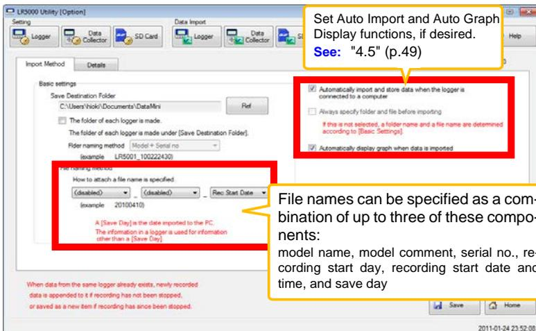
File names can be specified as a combination of up to three of these components:
