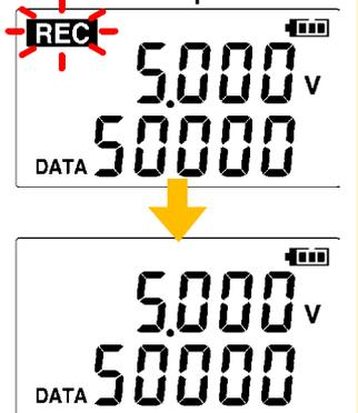
**Stop** Hold the **REC/STOP** button for two seconds while recording (while **[REC]** is displayed).
