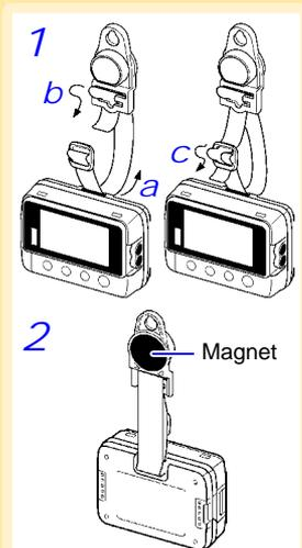
1 Attach the Z5004 to the strap/stand attachment hole.
