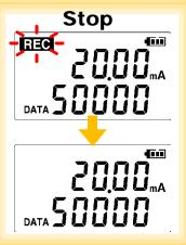
**Start** From the Measurement display, hold the **REC/STOP** button for two seconds.
