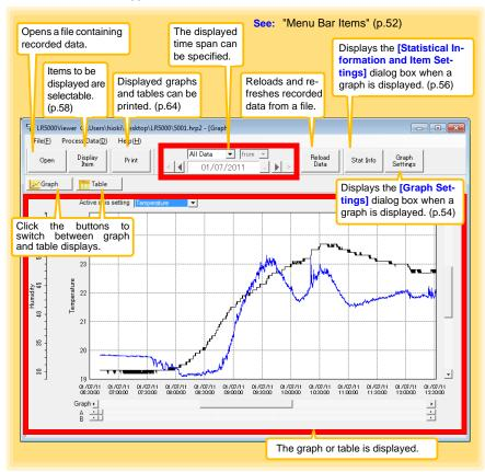
4.5 Automatically Importing (Saving) Recorded Data to a Computer, and Graph Display
