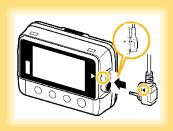
Align the triangles on the plug body and in front of the connection cable jacks, and insert the plug securely.
