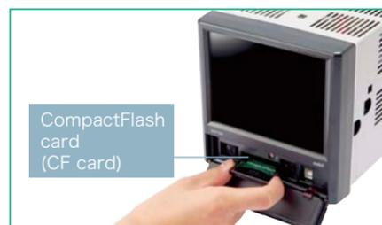
Front CompactFlash card slot. Data can be backed up "as is" to a PC.
