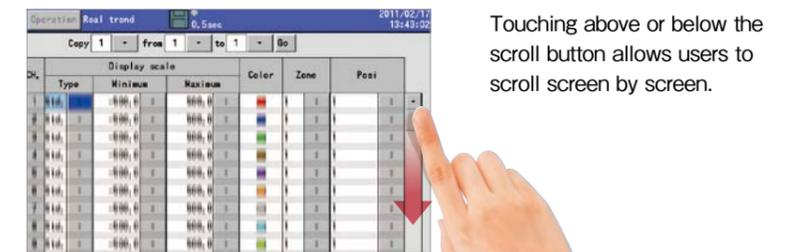
Touching above or below the scroll button allows users to scroll screen by screen.
